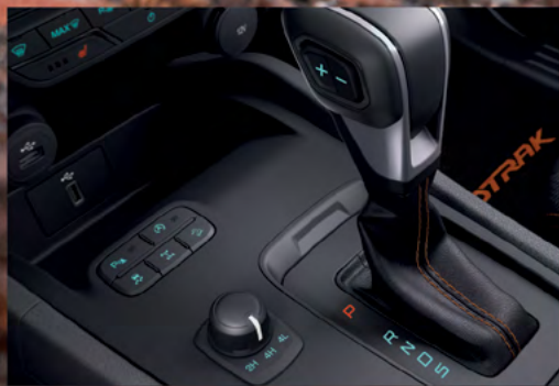
4x4 Drivetrain with Electronic Shift-On-The-Fly Mechanism
